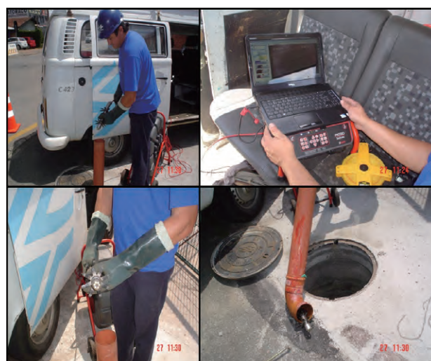
Field Investigation by Insert-Type TV Camera
