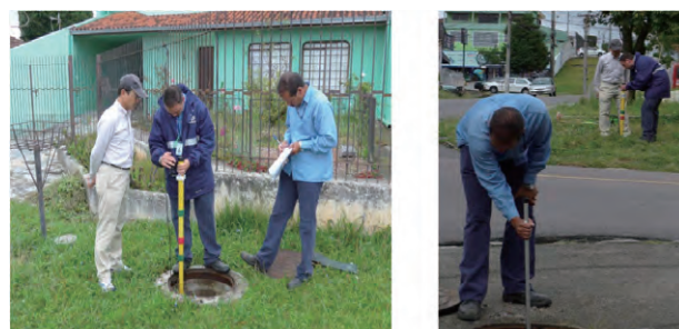
Field Investigation by Simple TV camera
